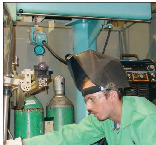
EWI technician sets up a GMAW torch powered via a MELTRIC Switch-Rated plug and receptacle.
