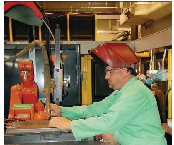
Welding technician Tim Moore prepares a GMAW torch on a mechanized fixture.
