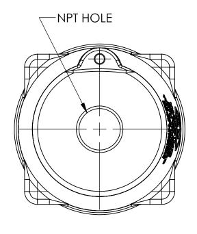
For use in Class I or II Division 2 or Class 1 Zone 1 or Zone 21 depending on fitting used. Fitting manufactured by others.
